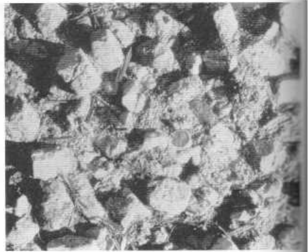
FIGURE 4: Weathered rock surface of Cathedral Peak Granodiorite with resistant feldspar crystals protruding above surface of more readily removed rock matrix. Penny provides scale.
